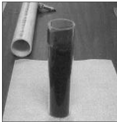
Figure 6. Photograph of the displacer prior to assembly. Note the acrylic cylinder which forms the displacer shell holds a bar magnet and the steel wool which composes the regenerator. The acrylic shell forms a slip fit inside the PVC tubing seen in Figure 5.
