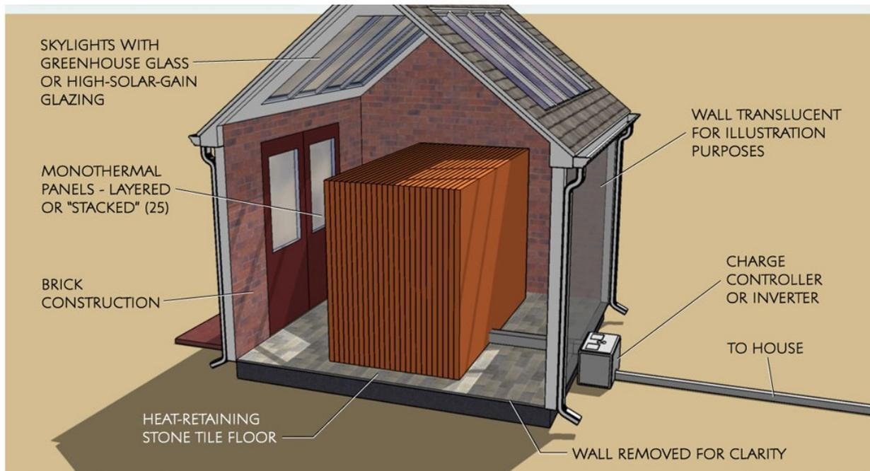
Panels can be designed in stacks that produce power for homes. The panels can be placed in a shed with greenhouse skylights adjoining the building. 25 panels can provide 35 kW during the warm part of a day and continue to provide some power all night.
